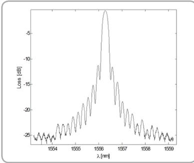
Fiber Bragg Gratings (FBGs) are widely used in the area of the sensing systems, telecommunications and in the other areas where the optical signal filtering is required. FBGs are produced by the lateral exposure of the optical fiber by the UV excimer KrF laser through a phase mask. We offer FBGs in the area of 1310 nm (O-band), 1520 nm (S-band), 1550 nm (C-band) and 1600 nm (L-band).
