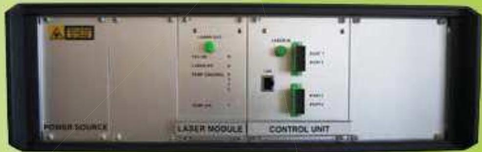
**Figure 2** Interrogation system with built-in broadband light source, spectrum analyser and four FBG sensor multiplexer
