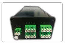
MEMS optical switch based on electronically driven micro-electromechanical system. The MEMS switch consists of an electrically control mirror on a silicon substrate. A voltage applied to the MEMS chip causes the mirror to rotate, which changes the coupling of light between the input and output fibers of the MEMS Optical Switch. 16 switching channels.
